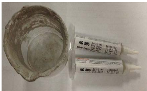
Figure 5. Silver epoxy-based ink (AG 806) produced by Penchem Technologies.
